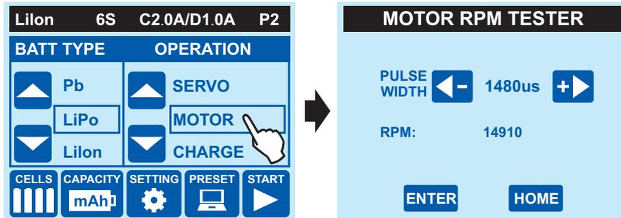
7. Switch on the ESC. Touch  $\leftarrow$  /  $\rightarrow$  to change the value of pulse width and check the RPM of the motor corresponding to different pulse width. If the motor doesn't run, please recheck the transmitters' neutral position and reset the initial pulse width.
