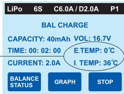
E.TEMP=External Temperature (Battery Temperature)
