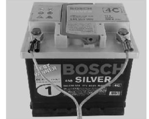
Using terminal clip attaching to car battery
