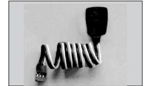
Temperature Probe with Magnet
